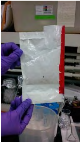
Figure 3: PresSure Lok bag with makeshift side support before incubation.
