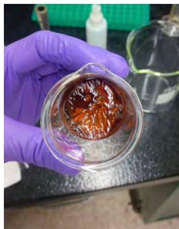
Figure 12: Media sample after two days in a 60° C vacuum
